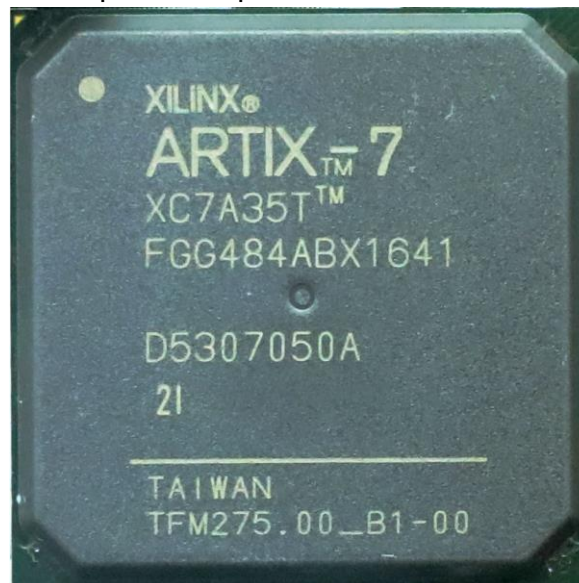
Figure 4-1: The Specific Chip Model Definition of ARTIX-7 Series
